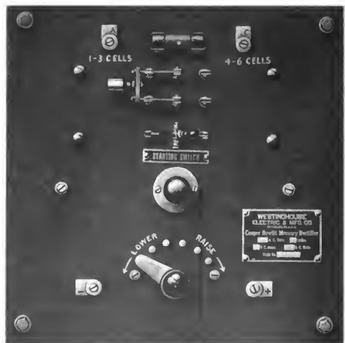
Type E Mercury Rectifier for Charging Ignition Batteries.
